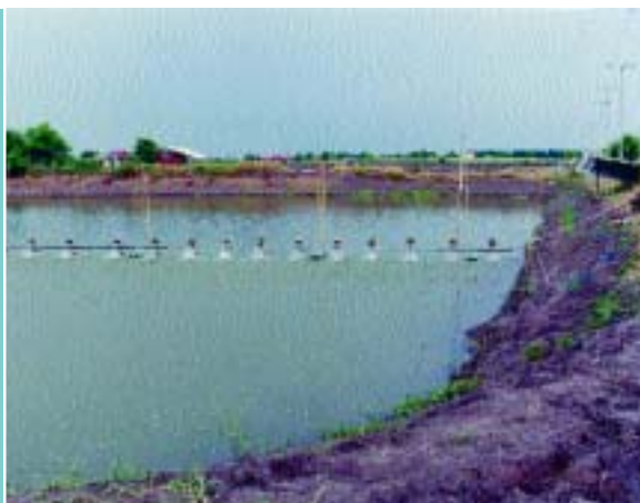
Figure 64 Long-shaft aerator in action (Thailand)
